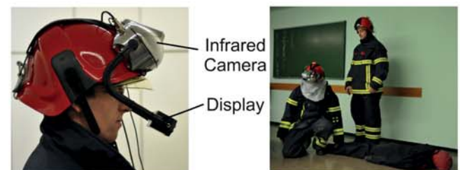
Figure 4: Left: Helmet-mounted Infrared Camera and Display. Right: Professional fire-fighters testing the system during a Profitex workshop (kneeling fire-fighter is blindfolded to test the navigation system)
