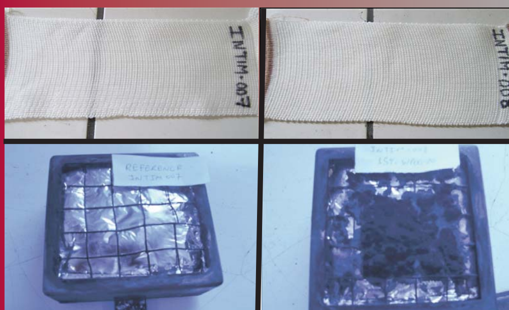
Fig. 4 - Knitted samples before and after cone calorimeter test (left, virgin PP; right, PP + 15 wt.% INTIMIRE additive)
