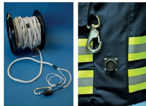
Figure 2: Left: Smart Lifeline v1. Right: Connection port in fire-fighting jacket
