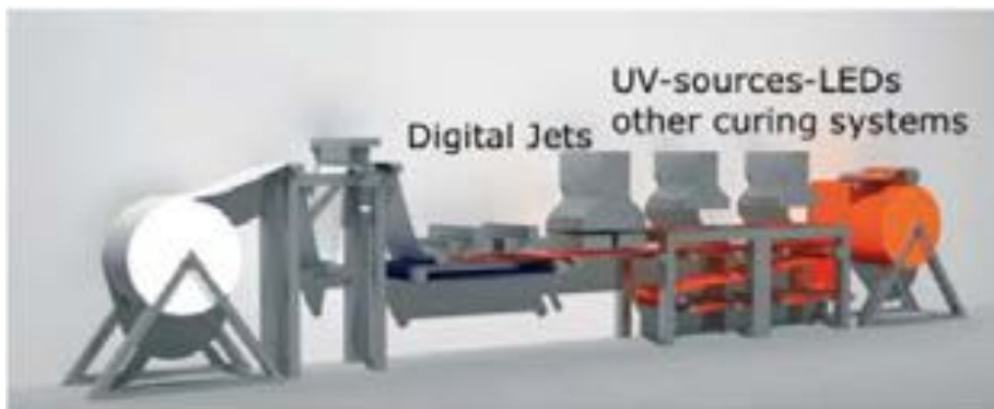
Figure : future coating processes based on digital coating and in-line UV-LED curing unites (EU-project Digitex)
